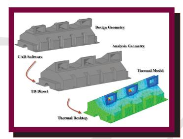
CRTech TD Direct® is devoted to the defeaturing, meshing, and preparation of CAD models for thermal analysis. Bi-directional linking provides synchronization between TD Direct and Thermal Desktop.
