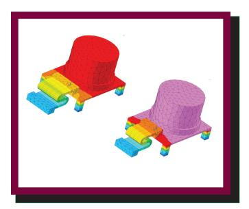
Evaluating the effects of reducing the width of a thermal strap using the integrated design process of TD Direct.
